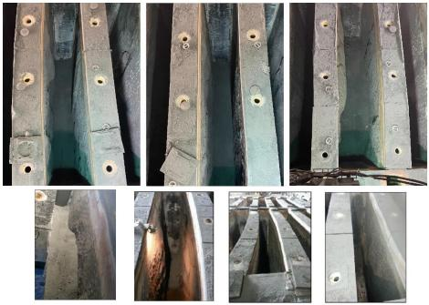
Figure 1. Different modes of pit deformations.
